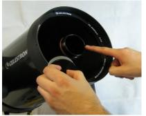
Set the Secondary Mirror into the telescope at an angle to prevent scratching the mirror
