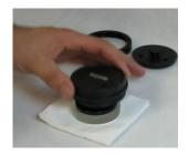
Set on the new Mirror Mounting Plate with the Index Mark in the correct position
