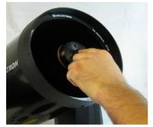
o Replace the Secondary Mirror Retaining Ring but do not over-tighten it
