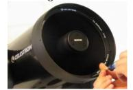
Careful removal of the retaining ring without touching the corrector plate
