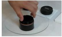
Align the Index Mark on the Corrector Plate with the notch in the Secondary Mirror Holder and begin to tighten the assembly
